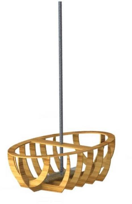
Figure 1: Render created in SolidWorks of the boat assembly. Includes models for the hardboard rib construction, the mast, and a place-holder for the ballast.
